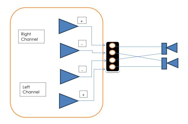
A Standard Class AB amplifier may work in this mode as the –v terminals are normally joined internally
